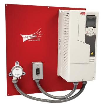
The Intelli-Blower control panel for use with Micro Air dust collection system that enables the dust collector to continually operate at the static pressure set point. By operating at the exact specifications your application requires, there is no wasted horsepower or energy. Once set up, the system will run at a constant CFM regardless of the changing static pressures or filter loading in the dust collector.
