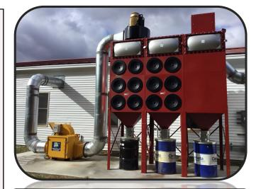
RP6-2 with Top Mount Fans with Drop Out Chamber (DOC) and XP Vent and OSHA/NFPA Combustible Dust Compliance Package
