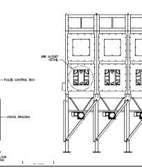
FRP8-3 EQUIPPED WITH REMOTE MOUNT FAN / LONG LEGS / HOPPER / INLET PLENUM / XP VENTS
