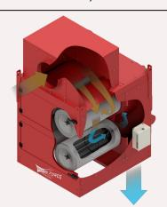
filter section, where the contaminant is filtered and dropped into the hopper or dust drawer. Breathe Easy, clean safe air is exhausted out the bottom of the unit. Cartridge cleaning is accomplished with Micro Air's proprietary Roto-Pulse® cleaning system, where air is pulsed
