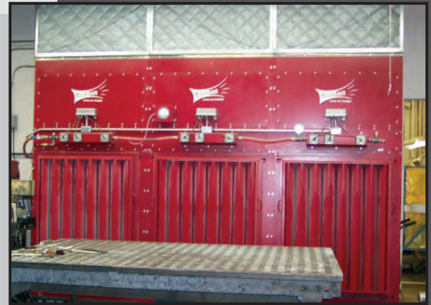
3-Module Clean Air Booth in Welding Operation
