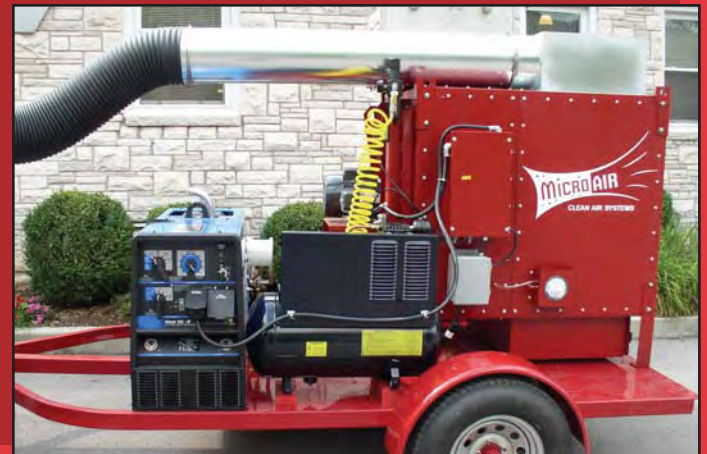
Trailer mounted RP4 collects cement dust
